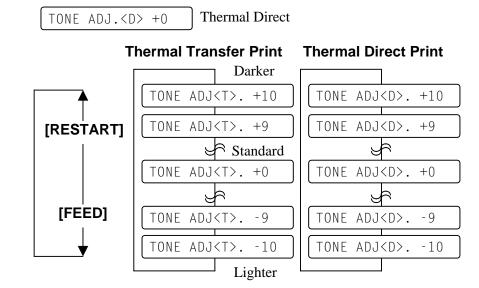
**[FEED]** key: Pressing the **[FEED]** key one time causes a -1 tone change, up to -10 tones.
